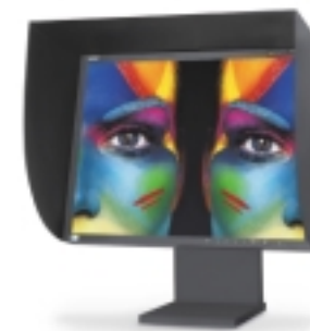
The hood serves as a 'digital dark-room', blocking out unwanted ambient light.
