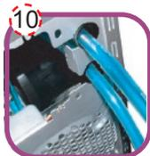
Rear retaining holes for liquid cooling kits
