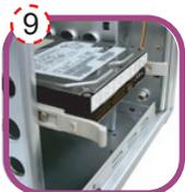
Screwless HDD for easy access
