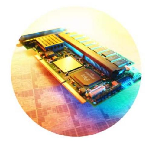
The Intel® RAID Controller SRCU42X, a PCI-X, dual-channel, Ultra320 SCSI RAID controller based on Intel® XScale® technology.
